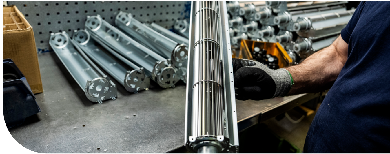
Assembly of crossflow blowers, FNE, Sweden
